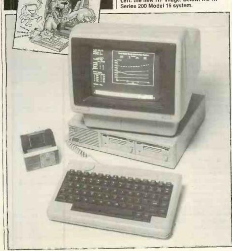
Model 16's Basic, which is typical of the whole HP approach, is that the same set of plotting and drawing commands work on a wide range of different output devices. With our set-up we could display the same graphics image on the screen, on the plotter or on the matrix printer simply by including a line of code to specify the device type.
